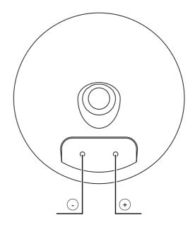
, Speaker input terminals When connecting the speakers, insert the ends of the speaker cables so that they do not touch neighbouring terminals.
