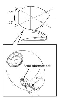
1 Use the Allen key which is supplied with the speaker to loosen the angle adjustment bolt underneath the speaker.
