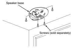
9 Install the speaker base at the speaker installation position using the screws (sold separately).
