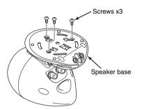
1 Remove the screws from the bottom of the speaker base.
