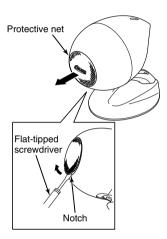
Insert the end of a flat-tipped screwdriver into the notch of the protective net, and lever it upward to lift up the protective net.
