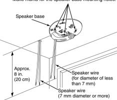
Use the speaker base to determine the speaker installation position on the ceiling inside the room, and then use an awl or similar tool to mark the positions of the speaker base mounting holes on the ceiling.
