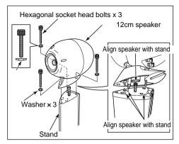
For the installation, insert the washer so the convex surface is facing down.
