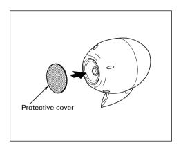
As shown in the diagram, install the protective cover.
