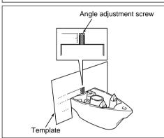
Turn the speaker base upside down and adjust the angle adjustment screw to a height matching the gauge as shown in the diagram. At this point, the angle is set at 0 degrees.
