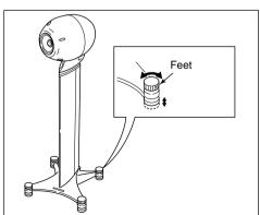
As shown in the diagram, turn the feet to adjust.
