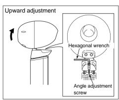
Using the hexagonal wrench, loosen the hexagonal socket head bolts (3 places).
